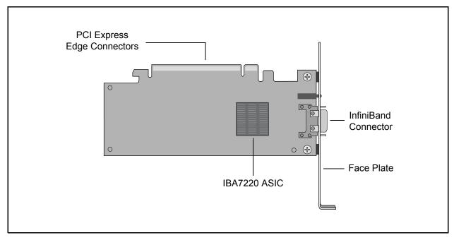
Figure 4-1. QLogic QLE7280 with IBA7220 ASIC
